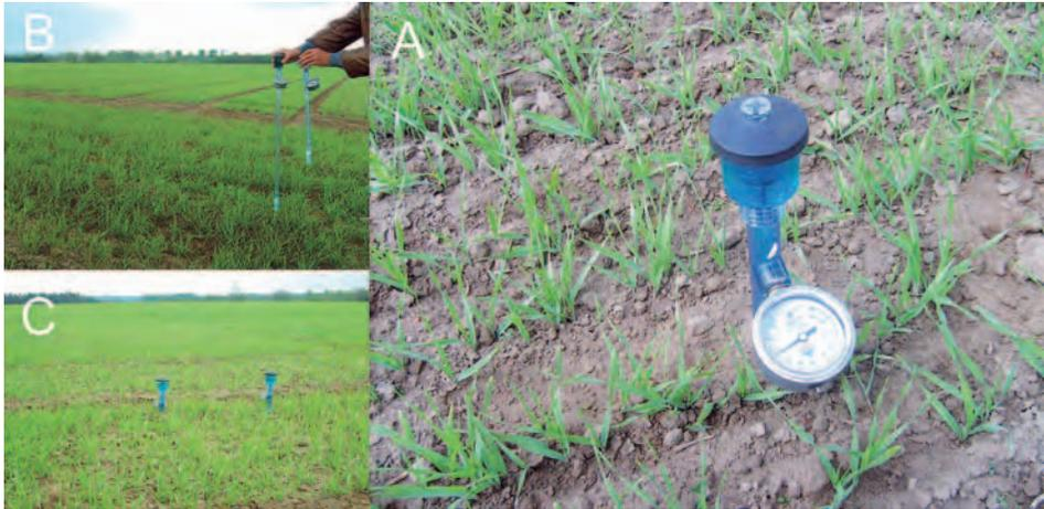
Fig. 5. Tensiometers (A) for two depths, 30 and 60 cm, installed in the field of spring barley (B, C)
