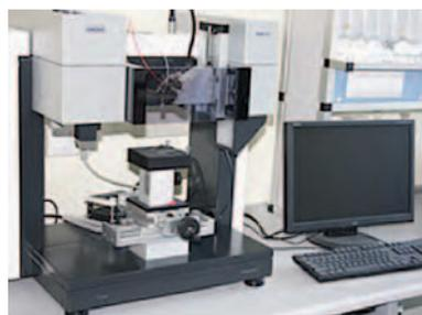
Fig. 8. KRÜSS drop shape analyser
