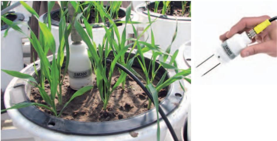
Fig. 13. SM300 Soil moisture and temperature sensor
