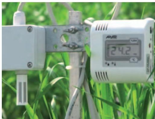
Fig. 4. Air temperature and humidity recorder
