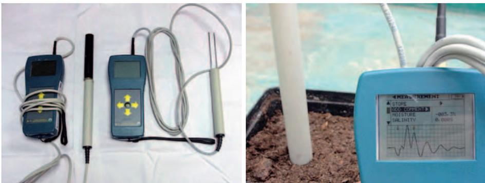
Fig. 7. FOM/mts – hand-held device designed for field measurements of soil moisture and temperature
