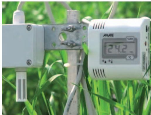
Fig. 4. Air temperature and humidity recorder
