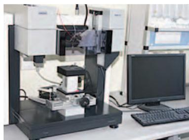
Fig. 8. KRÜSS drop shape analyser
