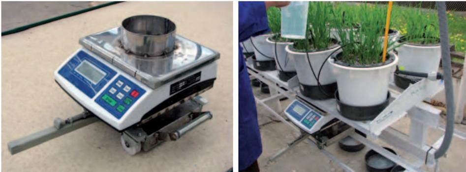
Fig. 14. Weighing control of soil moisture status in pots
